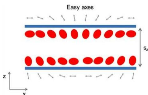
*Cartoon of confined liquid crystal. Anchoring conditions (easy axes) at the substrates vary periodically along the  $x$ -direction. Easy axes may be out of phase (shown); the period of variation may differ between the two substrates (not shown).*
