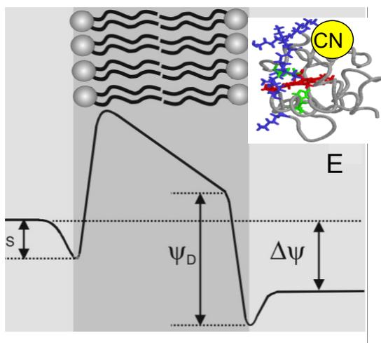
*Fig. 1. Incorporation of VSE reporter groups at different positions of the SAM/protein interface allows determining the local electric field.*
